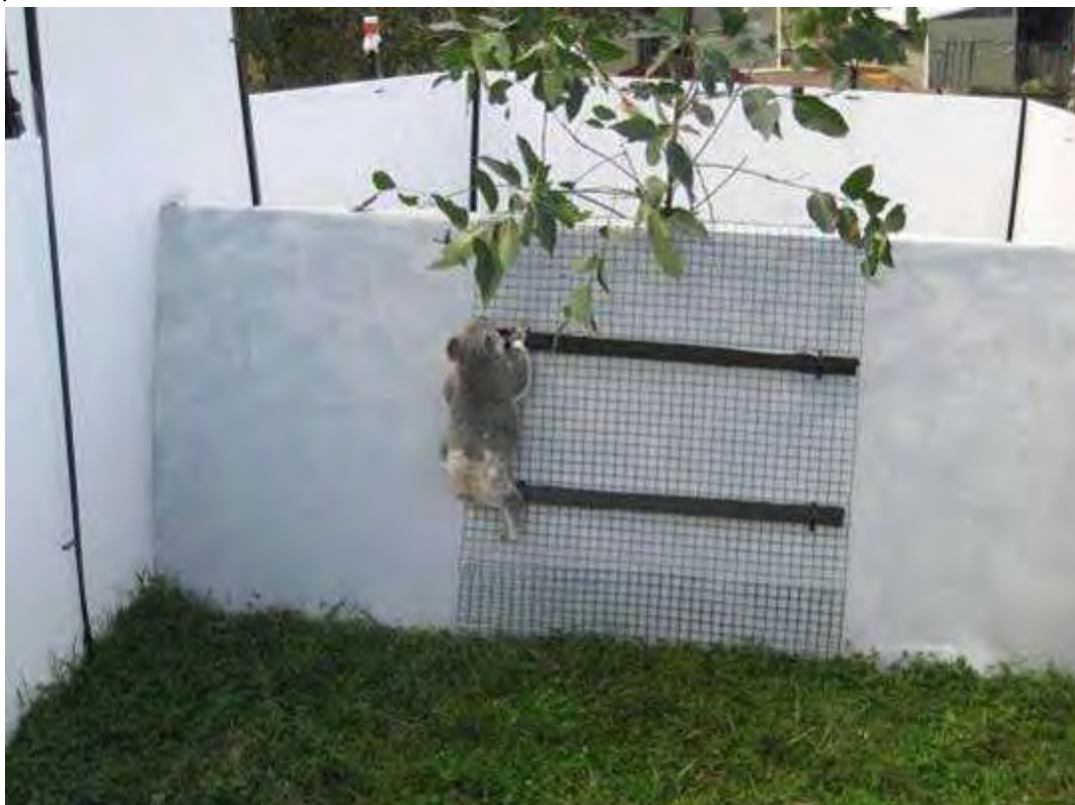
Figure 6.18.12 Koala barrier trials at the Australian Wildlife Hospital in Queensland. This koala was able to use wooden logs to climb over the simulated concrete barrier (Scott 2008).
